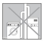
Note that to avoid condensation problems, it is essential that the dryer be fitted with the flexible hose to carry its "exhaust" at least beyond the kitchen units; preferably outside the kitchen.
